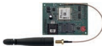
01706 Modul predajnika/prijamnika GSM Dual Band GSM/GPRS 900/1800 MHz
