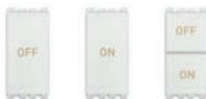
19056.33.B 10 A, kontakti 1 NO + 1 NC, OFF. Dubina: 29 mm 19056.34.B 10 A, kontakti 1 NO + 1 NC, ON. Dubina: 29 mm 19058.B Dva neovisna tipkala 1 NO + 1 NC, 10 A, simboli ON i OFF. Dubina: 29 mm
